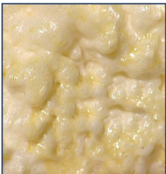
Off-Ratio, more "A" chemical is being dispensed
